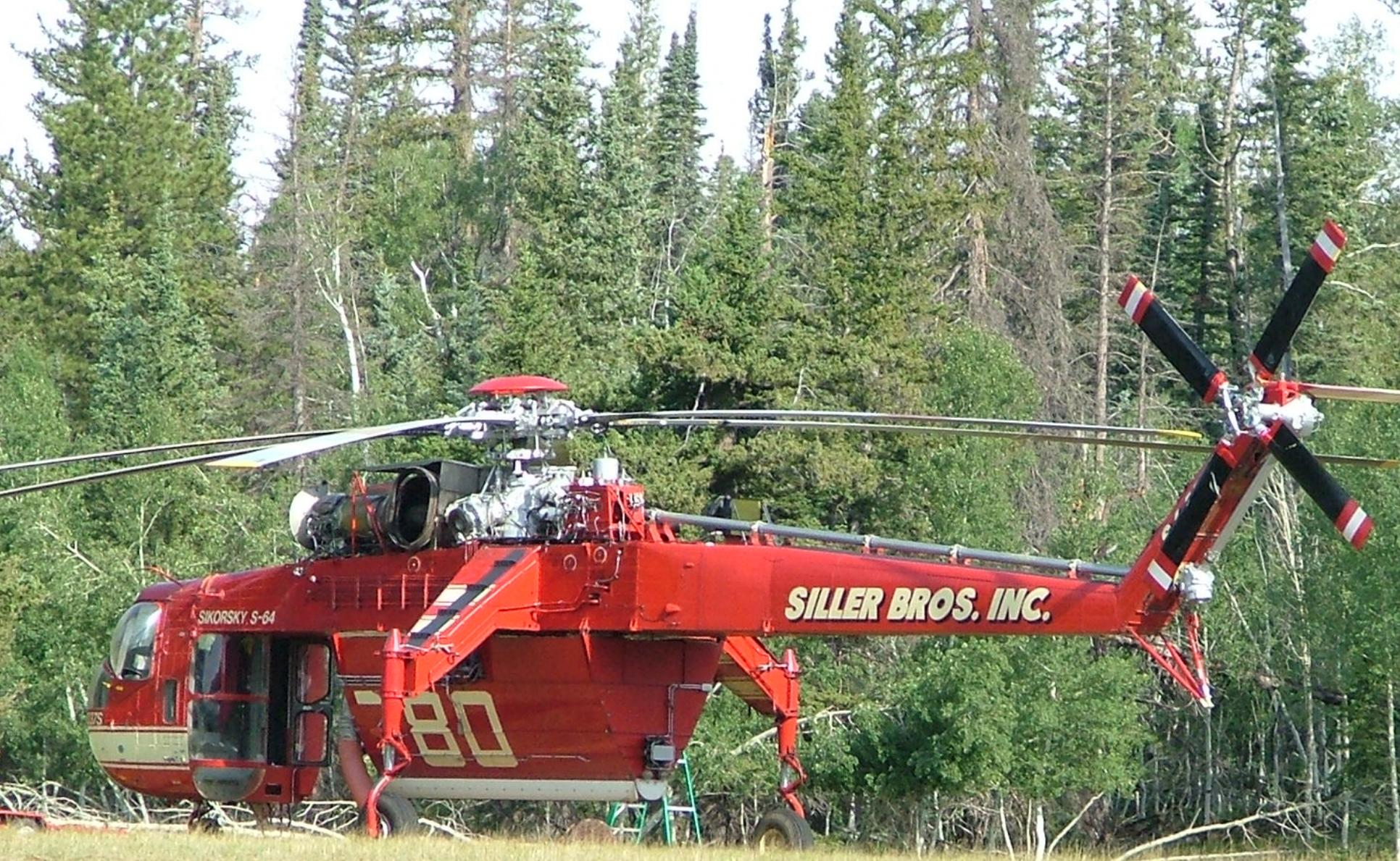
Ships- helicopters of various sizes can drop water or retardant. Also utilized to transport supplies, and crews into remote areas. Smoke, weather conditions can severely limit their use.
